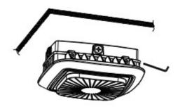
Close the fixture and fix the two parts with Allen Wrench
