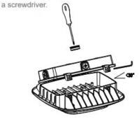
Get supply cord through the 3/4 inch hole, then attach driver box cover to ceiling and fix it with customer supplied hardware ,take relevant waterproof measures to make sure no water leakage.
