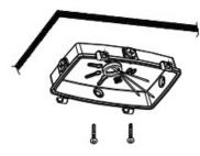
Hang the lamp to the driver box cover ,then let it fall naturally , connect the cord to the supply wiring . Set the dimming motion sensor if there is one.
