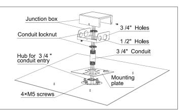
3. Place the mounting plate from above the ceiling, through the 4x M5 screws, and rotate the mounting plate and tighten the 4x M5 screws.4. Feed the luminaire wires through the 3/4" or 4" Conduit Rod, and make the connection on the junction box.
