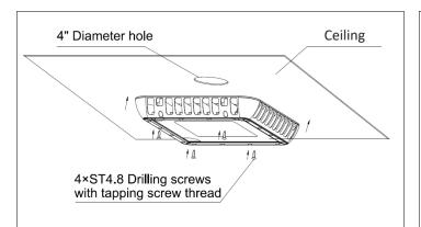
1. Cut 4 inch round hole at the center of the ceiling.
