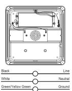
4. Disconnect the wires came from 3/4" hole and connect the wires came from 1/2" conduit with canopy.
