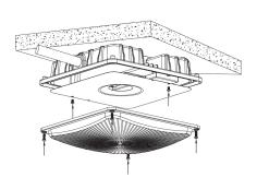
5. Replace the metal plate and the lens, make sure no wires are pinched when replacing parts.
