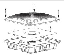
1. Remove the lens and metal plate by unscrewing the screws.
