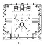
1. Loosen the screw on side of the light, removing the bracket from Canopy light by pulling it slightly out, just leaving the ring on bracket.
