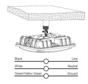
2. Connect the wires threaded from conduit and Canopy, Black wire for Line, White for Neutral, Green/Yellow Green for Ground.
