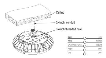
1. Connect the line voltage to the wires coming out from the fixture following the wiring diagram.
