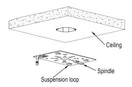
2. Fix the mounting plate to the ceiling with the screws.
