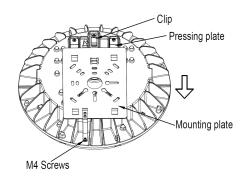
1. Loosen the screw on side of the light, removing the bracket from Canopy light by pulling it slightly out, just leaving the ring on bracket.
