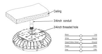
2. Screw the fixture to the 3/4 inch conduit to complete the installation.
