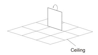
3. Rotate the panel light 90° in vertical direction to make it correspond to the recessed frame and be sure the front of the panel is facing the floor.
