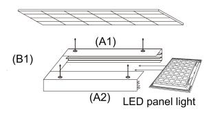
3. Secure A1 and A2 on the ceiling, and insert the panel light directly on the surface mount kit. Make sure the driver side is towards the opening.
