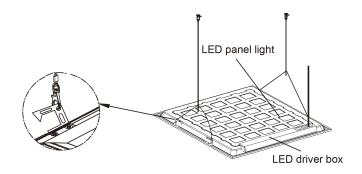
2. Install LED panel light by attaching the hook suspension wire to the metal brackets.
