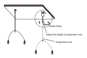
1. Install the suspension wire fixer on the ceiling, and make adjustment as necessary.
