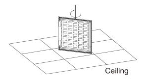
2. Rotate the panel 45° in horizontal direction to make the front of panel face the ceiling square hole.
