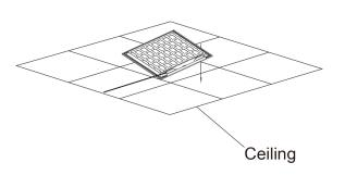
4. Pull the panel down towards the surface of the ceiling, and make adjustment as necessary to have it flush against the ceiling.
