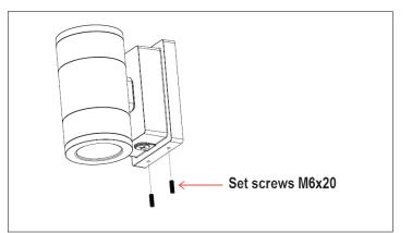
6. Secure the fixture on the wall by tightening the two set screws. NOTE: To ensure waterproof seal, apply weatherproof silicone sealant around the edge of the wall mounting box and/or junction box. This is especially important with uneven wall surface. Silicone all plugs and unused conduit entries.
