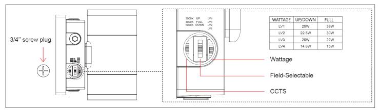
1. Remove the 3/4" screw plug to access the switch.
