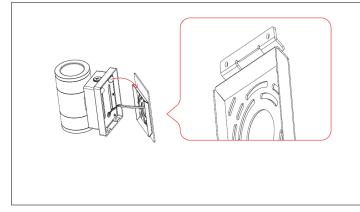
5. Attach the fixture to the mounting plate by sliding from the top.
