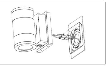
4. Make the wiring connection, according to the wiring diagram. Ensure Power is OFF prior to connecting wiring. CAUTION: Do not pinch wire
