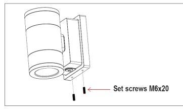
1. Loosen the 2 x set screws on the bottom of the fixture, to remove the mounting plate.
