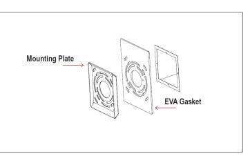
2. Install the EVA gasket to the junction box, and install the mounting plate over the EVA gasket. Make sure the holes of the mounting plate are align with the screw holes of the junction box.
